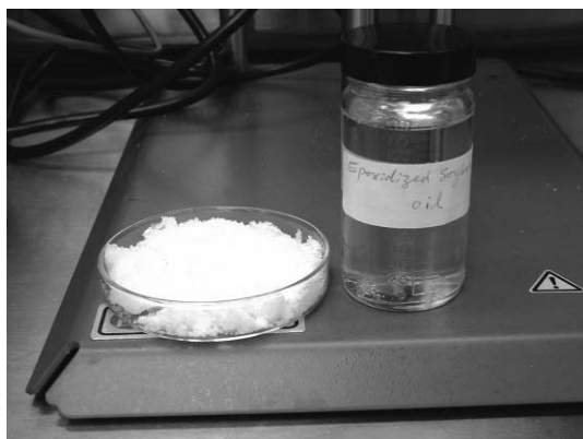
Fig. 3 Photo of RPESO polymers (dish) and starting material, ESO (bottle).
